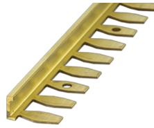
The stamped holes at regular intervals along the fitting strip serve as a means of additional attachment of the profiles using steel pins or screws along the planned, curved line. It is recommended that the profiles are first adapted to the desired radii and then bonded.
